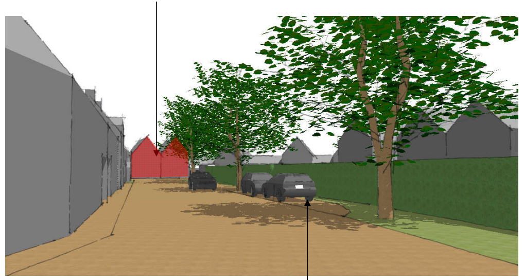
Visitor/additional parking can be provided on street, such as here in parallel bays 'book ended' by trees. Bays should be 6m x 2.4m.
